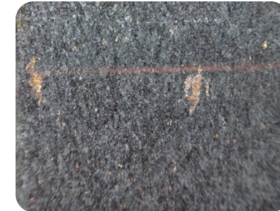
Sample No.: F1278 Visible Ni sulphide
